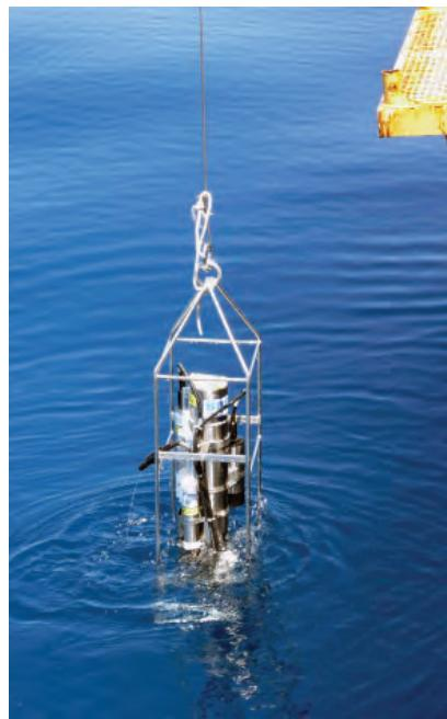
Slika 2. Mjerenje saliniteta, temperature i gustoće mora CTD (Conductivity-Temperature-Depth) sondom (Foto R. Garić).
