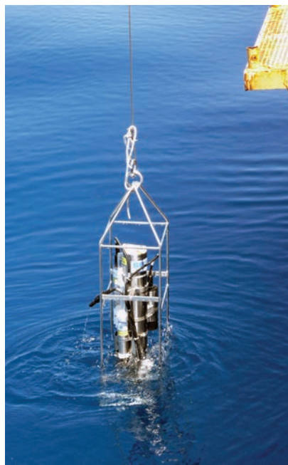
Figure 2. Measurement of salinity, temperature and density of the seawater with a CTD (conductivity-temperature-depth) probe (Photo by R. Garić).
