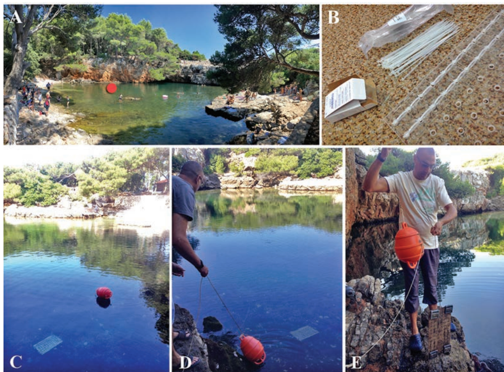
Figure 6. A – Location of the research station (red dot) in the marine Lake Mrtvo More ("Dead Sea") on the island of Lokrum off Dubrovnik in 2016. B – Plate with microscopic slides immersed in the Dead Sea at a depth of 1 m, C-E – Procedure for removing the plate with the microscopic slides to take a sample for diatom analysis (Photo by S. Ljubimir).
